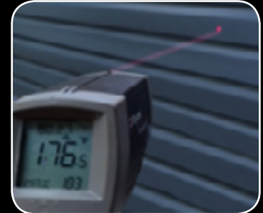
Heat gun pointed at Kaycan vinyl siding at a temperature of 176.5°F. No distortion from the intense heat.
